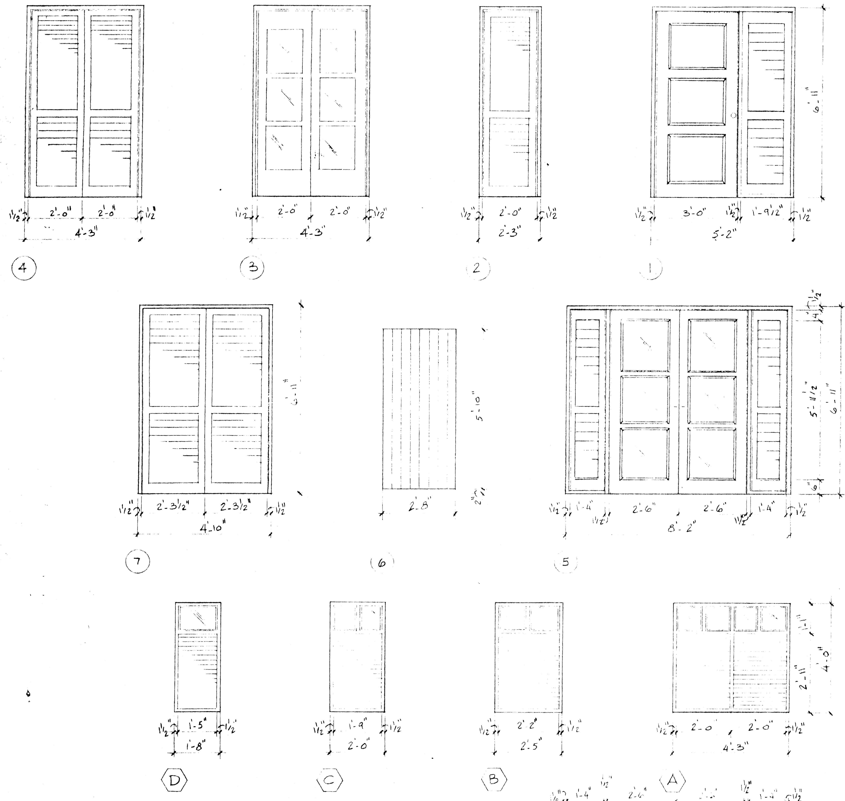
DOOR & WINDOW ELEVATIONS SCALE 1/2" = 1'-0"
